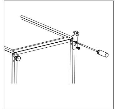
6. Unscrew and remove the bottom hinge pin with flat screw drivers, turn the bracket over and replace the pin.
