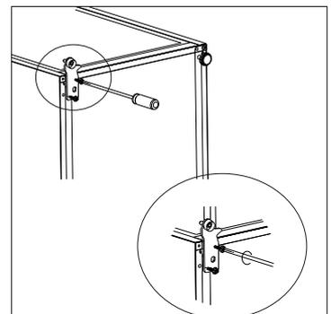
8. Place the door back on. Ensure the door is aligned horizontally and vertically so that the seals are closed on all sides before finally tightening the top hinge.
