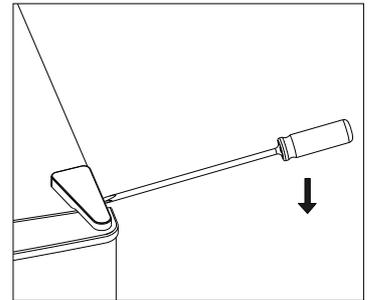
2. Undo the screws. Then remove the hinge bracket.
