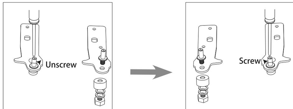
7. Refit the bracket fitting the bottom hinge pin. Replace the adjustable foot.
