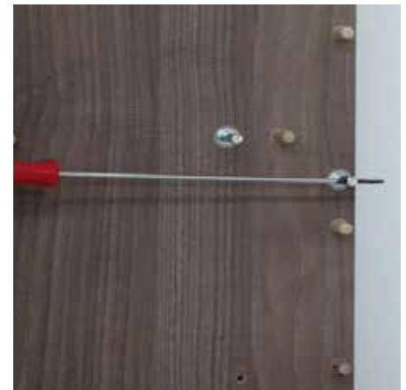
And the outside CAM PINS should be aligned in the horizontal position.
