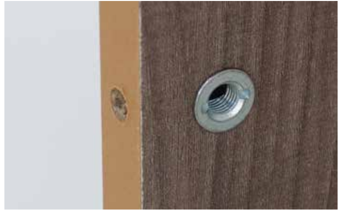
CAM in place with small indentations facing the CAM PIN .
